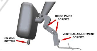
4 - Install the RD onto the mount. We recommend you adjust the RD so it is as close to the bottom of the mirror as possible. Using the vertical adjustment and orienting the double pivot center link, adjust RD upward as far as possible while making sure the mirror dimming switch is still accessible. After all adjustments are made, be sure to check that the pivot and vertical adjustment screws are tight. Grab the long arm of the allen wrench to assure that these screws are securely tightened.
