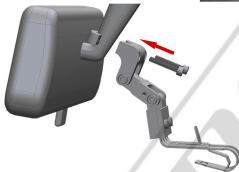
**3 - Install the mount while sitting in the passenger side of your vehicle.** Remove the two socket head screws so the top portion of the mount may be removed. Position the mount on the bottom of the stem as shown above. Reattach the top portion of the mount. Tighten both screws evenly making sure it is in the correct position as shown above. Tighten both screws until mount is securely attached to the mirror stem.
